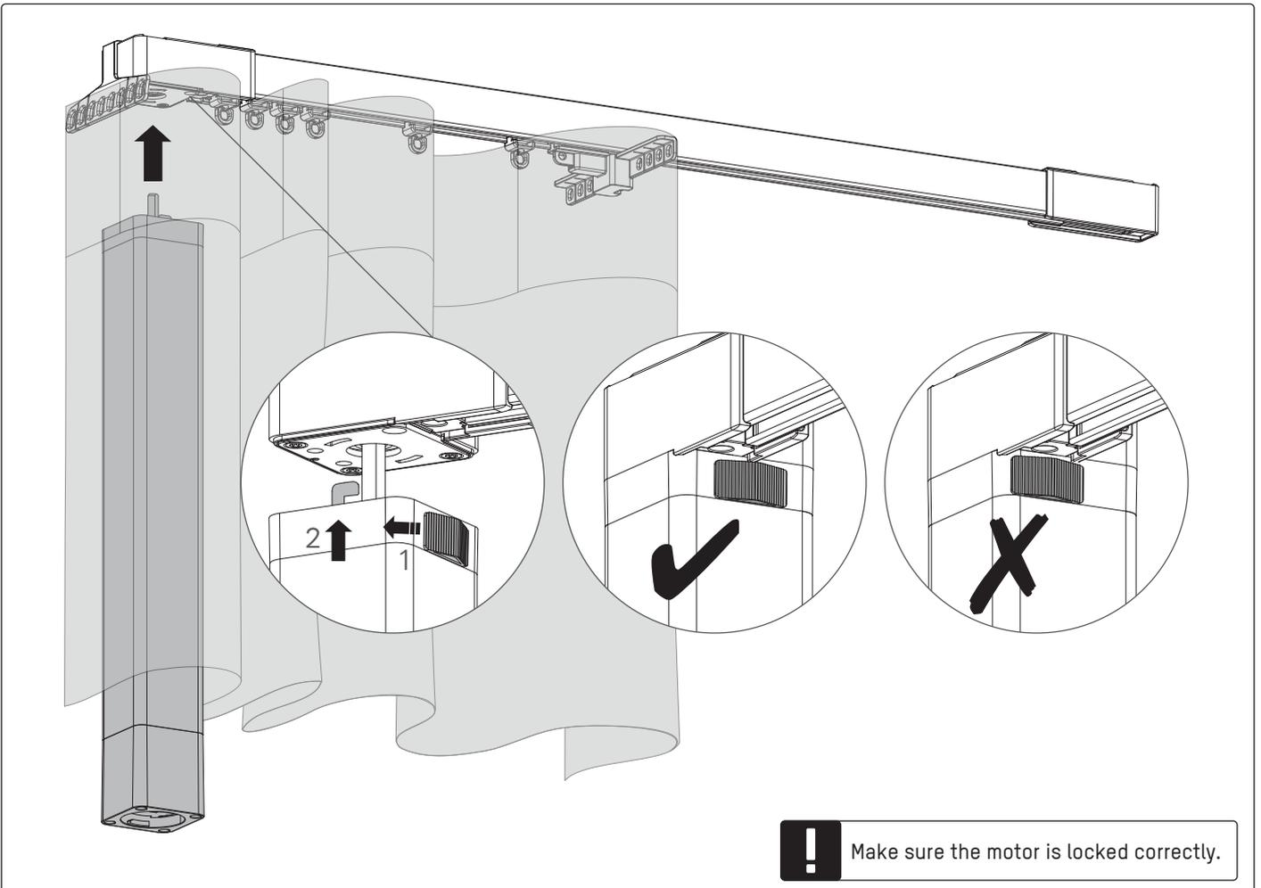
**!** Make sure the motor is locked correctly.
